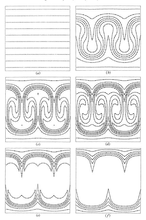
Figure 4. Expulsion of a horizontal field from a convective layer. Sequence with  $R_m=1000$ : (a) t=0.0, (b) t=0.5, (c) t=1.0, (d) t=1.5, (e) t=2.0, (f) t=3.0.
